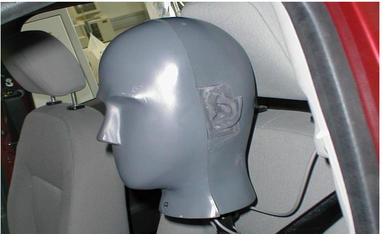
Image 10: Acoustic measurement set up in a car body by "Kunstkopf"
