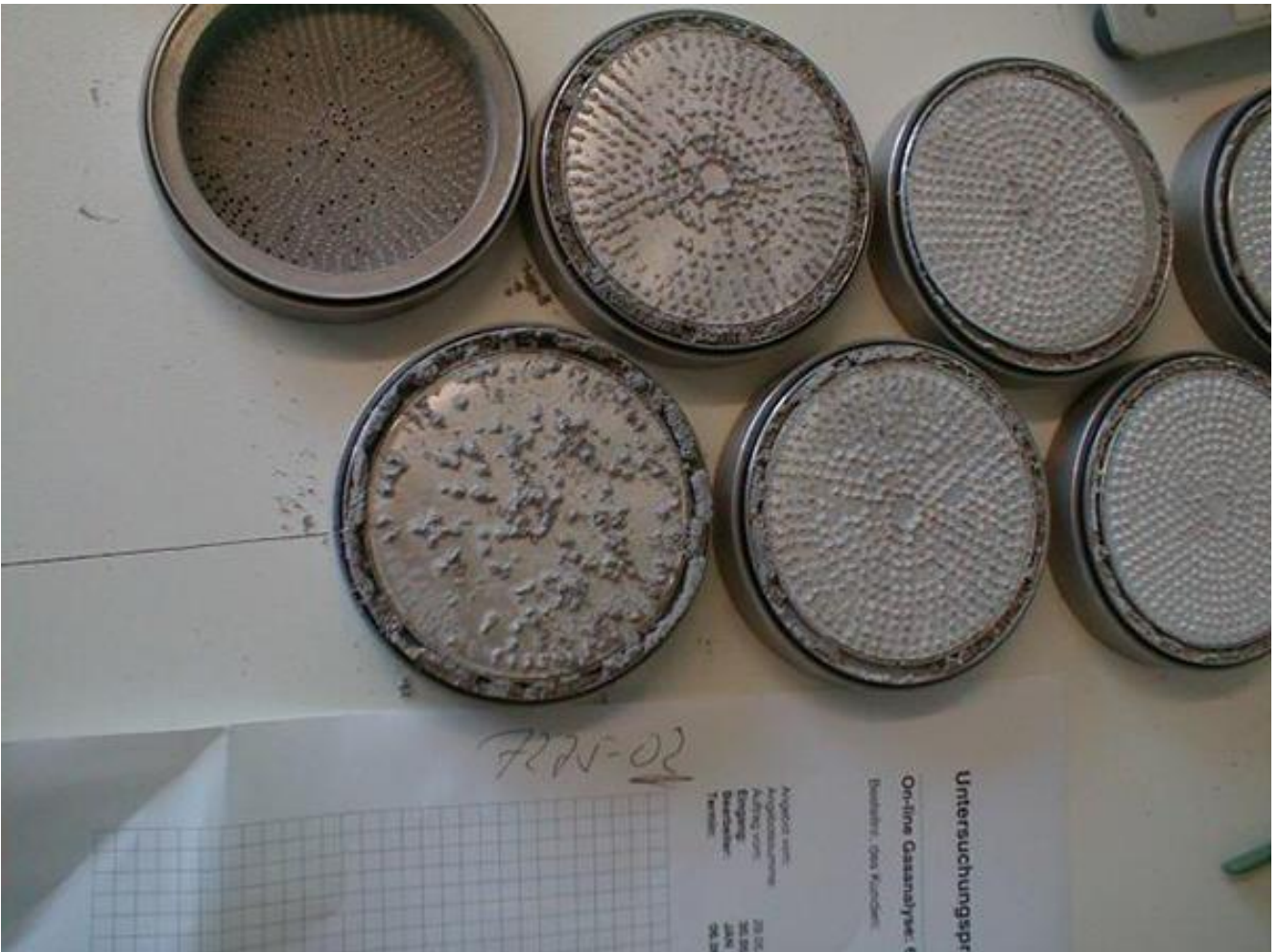
Image 6: Andersen impactor, example of overloaded impactation discs
