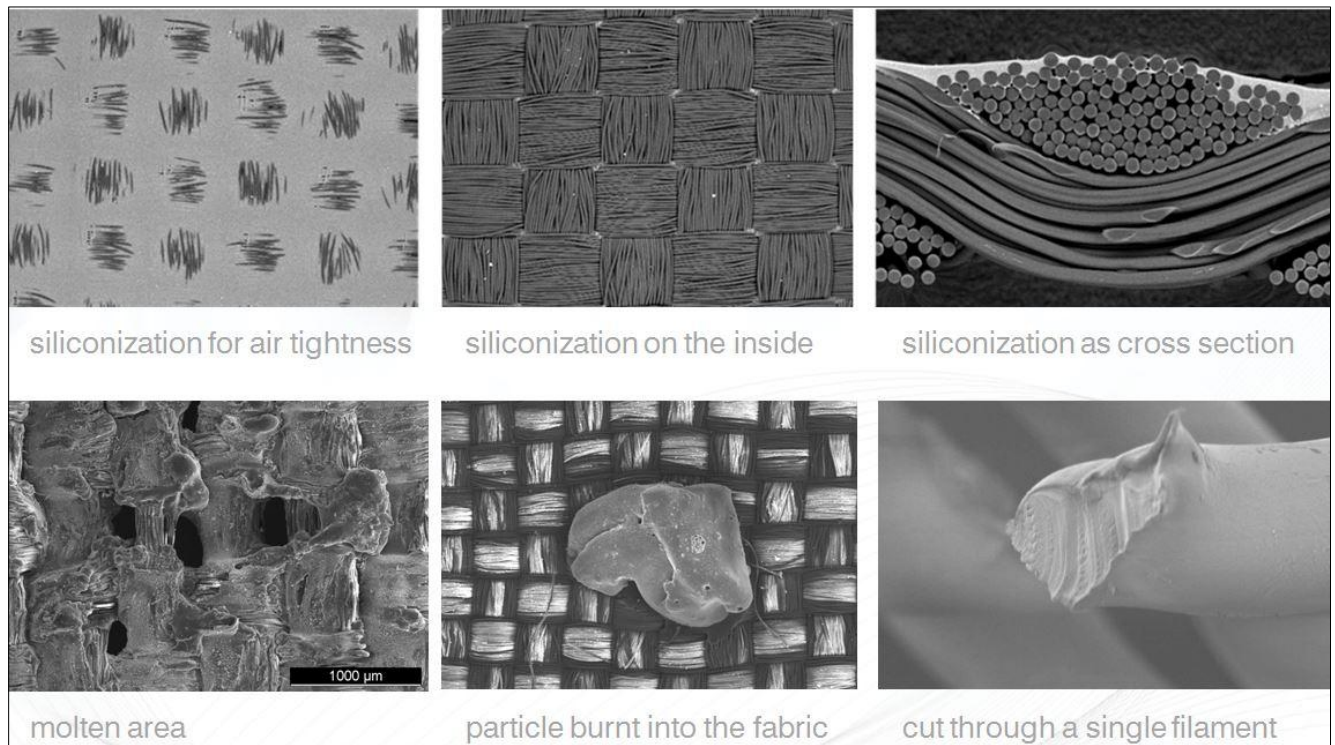
Figure 17: air bag fabric and possible defects
