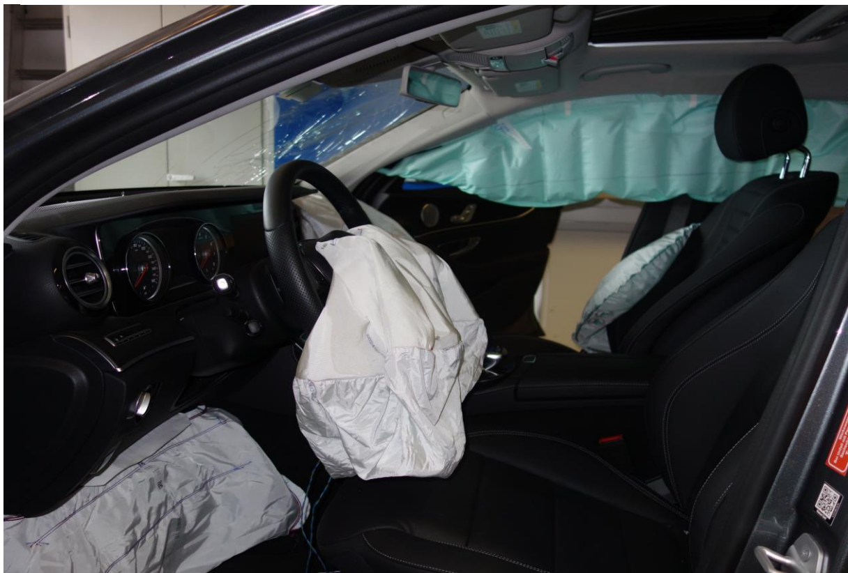
Picture 8: typical situation after complete airbag action
