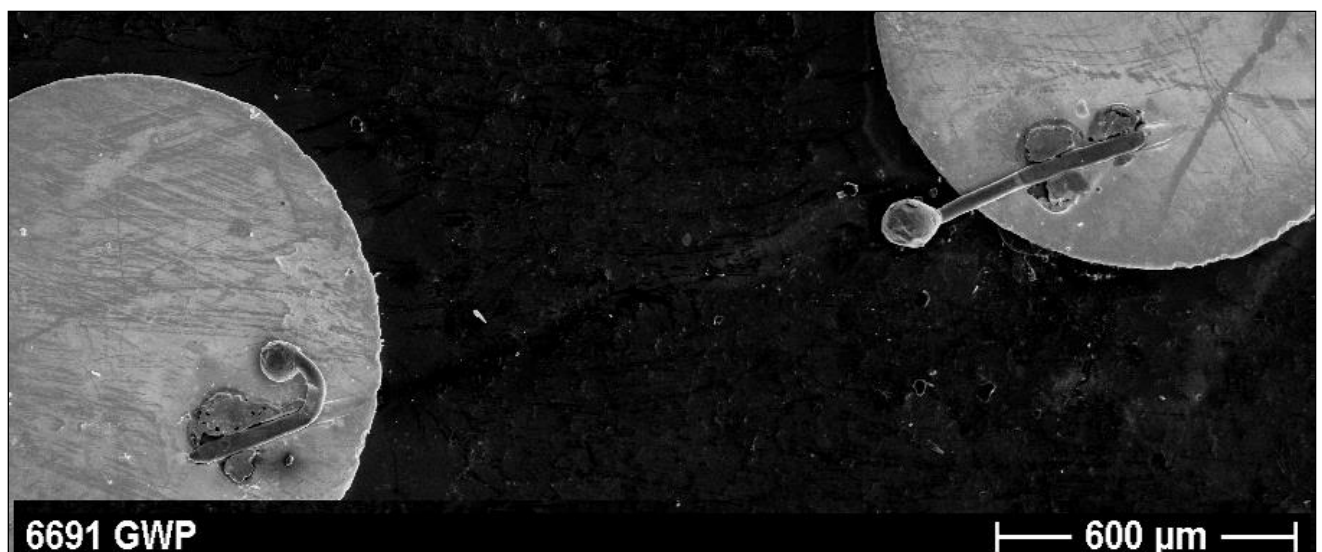
Figure 16: Molten filament (Glow Bridge).
