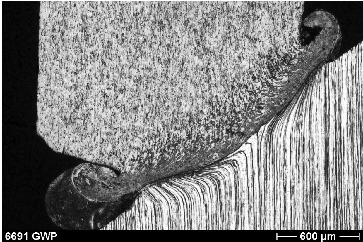
Figure 9: condenser discharge welding of the plug (above; ferrite steel) and cold gas cylinder (below; austenitic steel).
