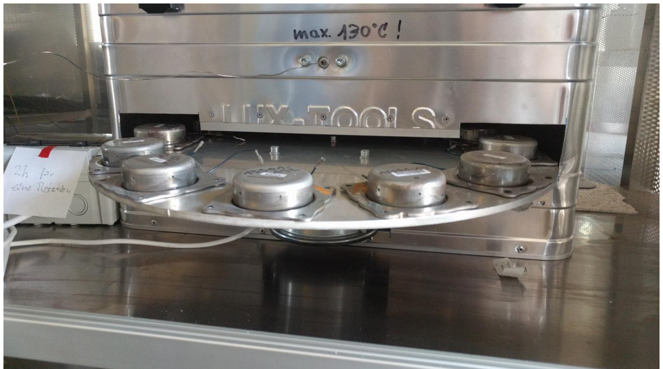
Figure 20: experiments for accelerated aging of components by thermal cycling for adjusting life cycle tests
