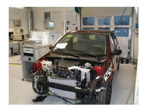
Measurement of emissions in the field of vehicle occupant restraint systems
